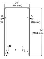
Cabinet depth frameless installation style = 25" (635 mm) Cabinet depth inset installation style = 25" (635 mm) + panel thickness
