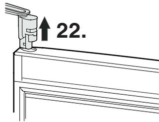
**22.** Using a screwdriver, push out the hinge from underneath and remove it from the door .
