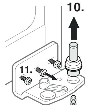
9. Tilt appliance slightly backwards and unscrew the adjustable foot.
