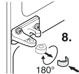
8. Remove hinge bushing, turn through 180° and re-fit.
