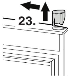
**23.** Using a screwdriver, push out the plug from underneath and transfer it to the opposite side.
