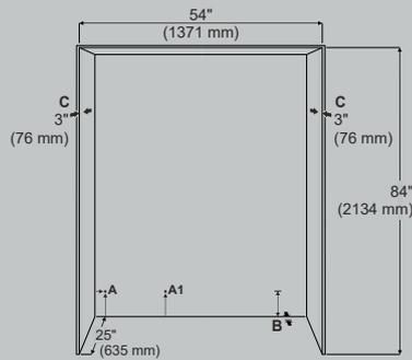
**A:** This is where the power cord exits the appliance rear, 3/4" (19 mm) from the left and 5" (127 mm) from the floor. Free length of the power cord is 98" (2.5 m). Power outlet is recommended to be placed outside of the appliance opening. A power supply of 220-240V with circuit grounded and protected by a circuit breaker is required. Socket must be properly earthed and protected by a fuse of 15A or 20A.
