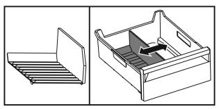
Fig. 113 Example illustration of the ice compartment divider
