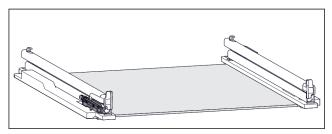
Fig. 129 Damping mechanism
