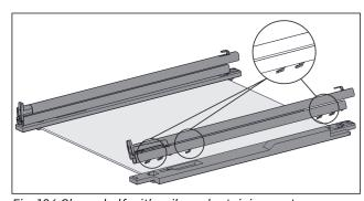
Fig. 126 Glass shelf with rails and retaining parts
