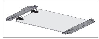
Fig. 127 Glass shelf with retaining part
