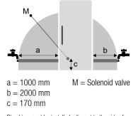
Plumbing must be installed adjacent to the side of the appliance which contains the IceMaker. Water pressure must be between 0.15 MPa and 0.6 MPa (1.5 bar - 6 bar)
