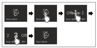
*Fig.* 35 *Example illustration: Change door alarm from* 1 *minute to 3 minutes.*
