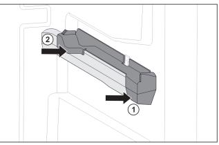
Fig. 63 Attachment on the right moulded rib
