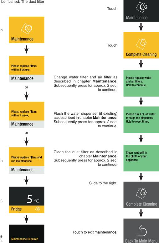
Obtain water filter and air filter from your dealer and complete the maintenance procedure.
