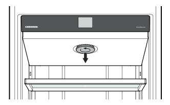
Turn the cover anticlockwise and remove it.
