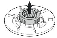
Insert the new air filter and turn clockwise until it snaps in.
