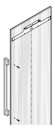
Only use countersunk screws for handle mounting.
