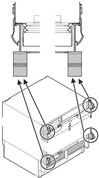
Recess Top view Slide the appliance into the recess. To avoid damage, move the power cord and the water line at once.
