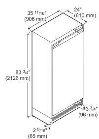
Stated minimum height dimensions include when the levelled feet are fully inserted. Width will increase by 1/4" (6.5 mm) when mounting strips are installed.
