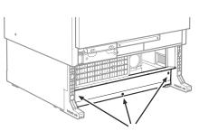
The steel plate can be removed to facilitate connecting the water hose.
