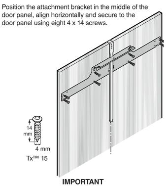
Risk of damaging the panel. Do not undershoot the minimum panel thickness (shaker style).
