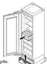
4. Remove the box with mounting parts.
