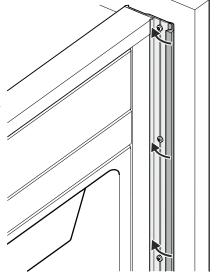
Push the mounting strip upwards. The bottom edge of the mounting strip must be aligned with the top edge of the adjacent cabinet door.
