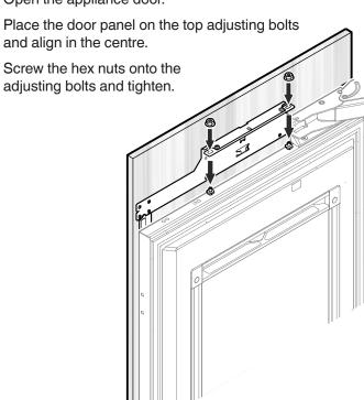
Close the door and check the position of the panel.
