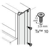
Apply the appliance cover strips to the left and right front edge of the appliance housing, align in height with the top profile and screw into place. The strip is transparent so the designed mounting holes on the appliance housing are visible. We recommend that you mark and predrill the hole positions in the strip.
