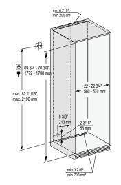
This is a fully integrated refrigerator appliance designed to be completely enclosed in a dedicated kitchen cabinet. This dedicated cabinet box must be constructed in accordance with the specified dimensions and must allow for sufficient air circulation to ensure proper operation. For more details about ventilation requirements, please refer to page 44.
