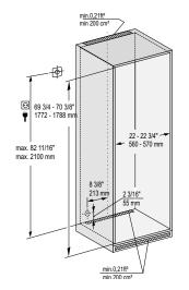
This is a fully integrated refrigerator-freezer appliance designed to be completely enclosed in a dedicated kitchen cabinet. This dedicated cabinet box must be constructed in accordance with the specified dimensions and must allow for sufficient air circulation to ensure proper operation. For more details about ventilation requirements, please refer to page 44.
