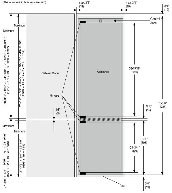
(a) The base of the cabinet can be thickened to raise the the top of the lower door panel to counter height. Lower panel will have to be increased in length by the same amount.
