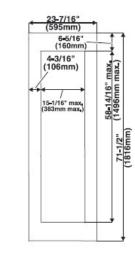
Custom panels should be at least 5/8"(16mm) and a maximum of 3/4"(19mm) thick and they should cover the front of the dedicated cabinet box.
