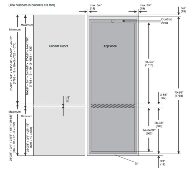
(a) The base of the cabinet can be thickened to raise the the top of the lower door panel to counter height. Lower panel will have to be increased in length by the same amount.
