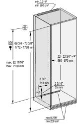
This is a fully integrated wine appliance designed to be completely enclosed in a dedicated kitchen cabinet. This dedicated cabinet box must be constructed in accordance with the specified dimensions and must allow for sufficient air circulation to ensure proper operation. For more details about ventilation requirements, please refer to page 44.
