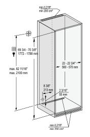
This is a fully integrated refrigerator appliance designed to be completely enclosed in a dedicated kitchen cabinet. This dedicated cabinet box must be constructed in accordance with the specified dimensions and must allow for sufficient air circulation to ensure proper operation. For more details about ventilation requirements, please refer to page 44.
