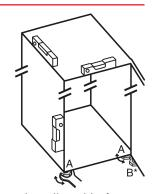
► Then prop up the door: Screw out the adjustable foot on the bearing bracket (B) using the open-ended wrench SW10 until it comes into contact with the floor, then turn an additional 90°.
