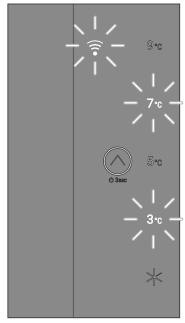
Fig. 46 Display in the event of a WLAN error
