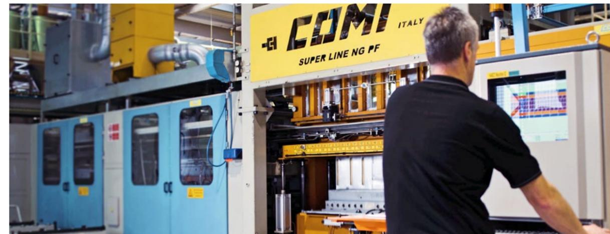
Thermoforming machine innerliner at the Ochsenhausen site
