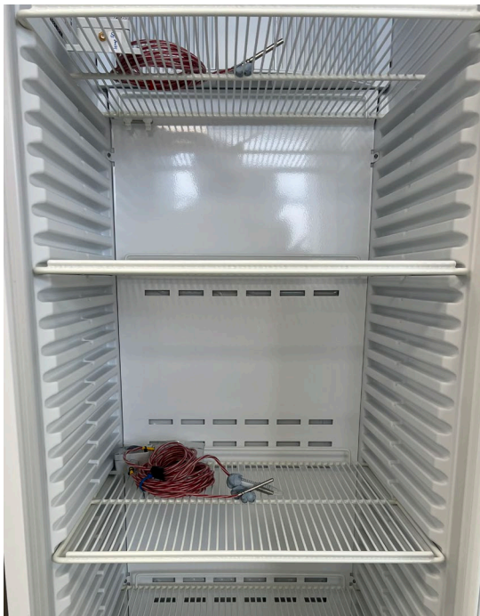
Figure 1. SRFvH4011 with probes positioned in the top compartment and middle compartment.
